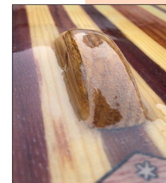
Leash cleat finished, mounted and under fiberglass cloth and epoxy resin.
